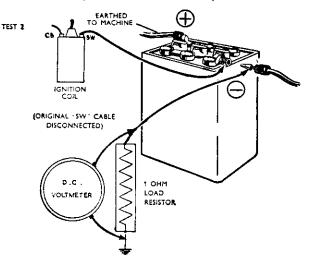
If battery is in poor condition or low state of charge use Test 2.
