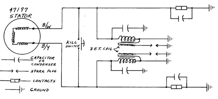
The stator windings must form a closed circuit (thru ground) in order that the rotor/stator can generate an A.C. voltage output. Remember a basic rule of electricity - electric current always takes the path of least resistance.
