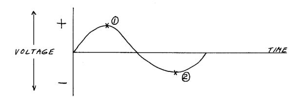
For maximum efficiency, the rotor/stator and the ignition contacts must be timed so that the points open very close to the point where the generated A.C. voltage is a maximum, i.e., points 1 & 2. This correct timing is assured if the rotor is timed to the engine crankshaft correctly.
