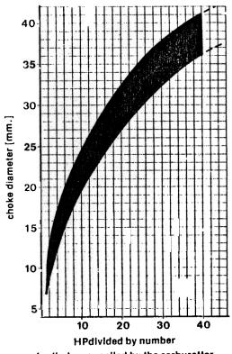
of cylinders supplied by the carburettor
